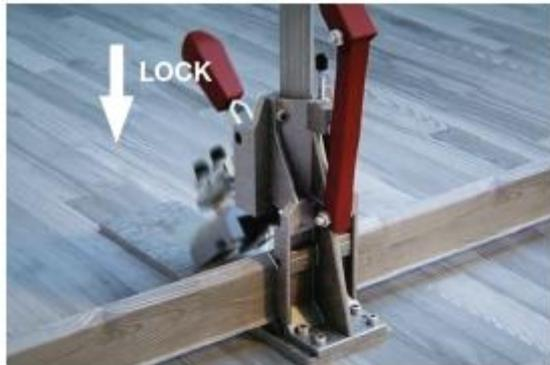
Lock the clamping device..
