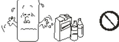
The volatilized chemicals might damage the unit and make the tank leak.
